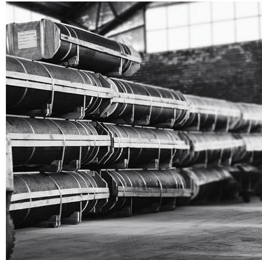
To produce graphite electrodes, needle coke powder is first molded and compressed with a vibrator. The formed electrode is then baked in an oven. After baking, a layer of bitumen is added to it. Finally, this product is again at a temperature of 3000 degrees Celsius and turns into graphite.
